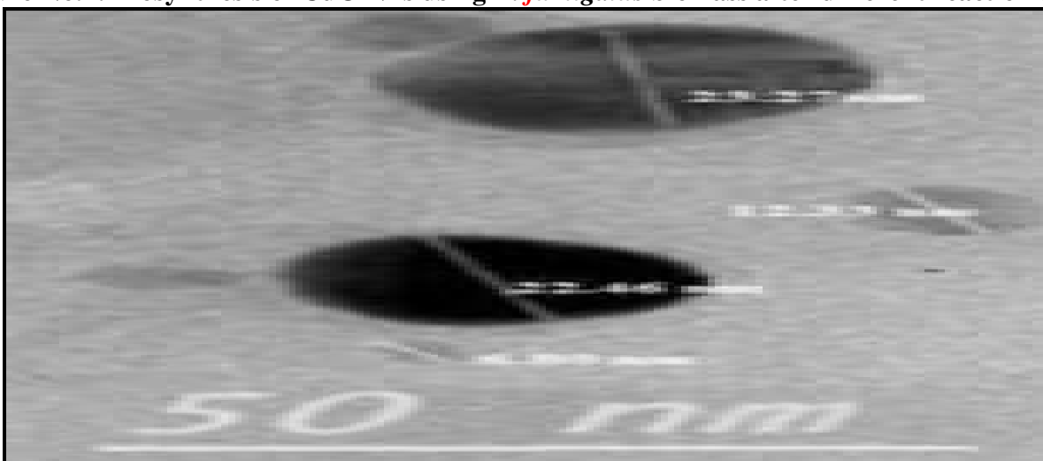
Figure No.5: TEM micrograph of CuO NPs biosynthesized using A. fumigatus preformed biomass from copper nitrate
